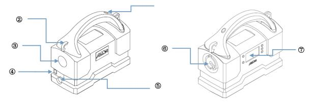
1.Switch 2.Strap holder 3.Air flow hole 4.Charging Socket 5.Valve adaptor 6.Inflation port 7.LCD Display
